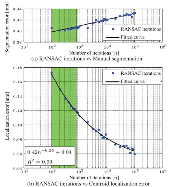
**Fig. 5.** Experimental evaluation and validation of image segmentation using a sequence of 600 ultrasound images. (a) Compares the performance between varying random sample consensus (RANSAC) iterations using a ground truth obtained by manual segmentation. (b) Describes the relation between the number of iterations and the localization error using a ground truth obtained after  $10^6$  RANSAC iterations.
